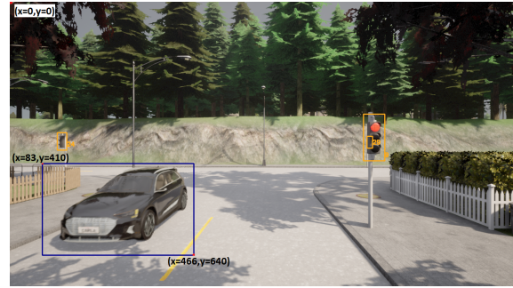
Figure 6: The coordinates of the box of an object are shown. We defined the corner coordinates of the box on the car as (x min, y min, x max, y max) = (83, 410, 466, 640) respectively.
