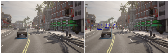
Figure 11: Labelling of bounding boxes up to 50m (left) and up to 100 m (right).
