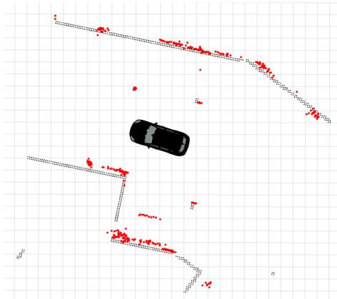
(a) Matching radar point clouds (red dots) to map data (black structure) for localization purposes
