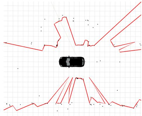
(b) Radar free space detection (red line) based on radar points (black dots)
