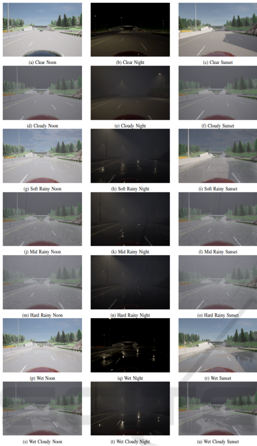
Figure 12: Overview of the generated dataset from SOTIF-related Use Case depicting diverse weather conditions.
