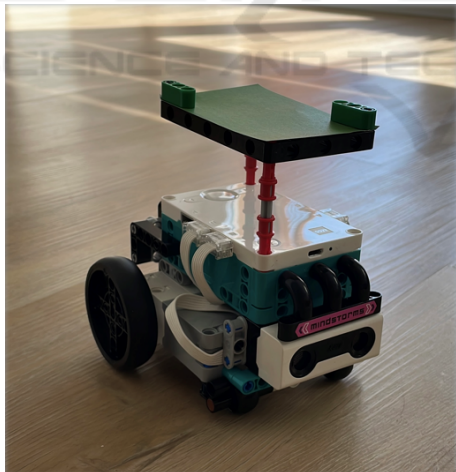
Figure 13: The robot used in the experimental part - based on Smart Element Hub cube with LED screen of the Robot Inventor kit.
