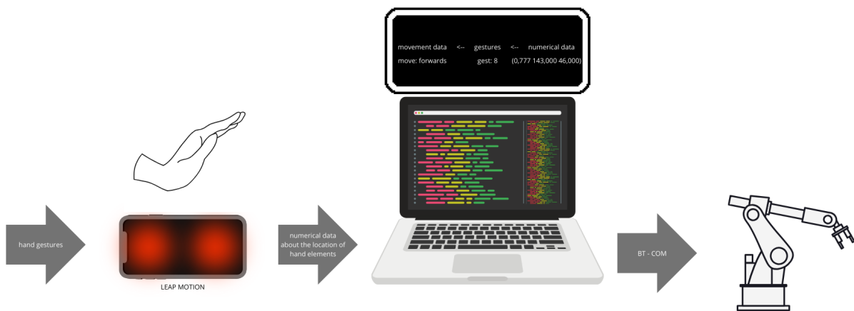
Figure 1: Graphical presentation of the system - use of Leap motion as a case study.
