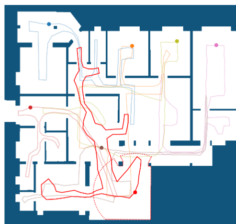
Figure 2: Visualization of the environment map, including starting points, exploration pathways and lidar range for the robotic agents, as described by (Yu et al., 2022).
