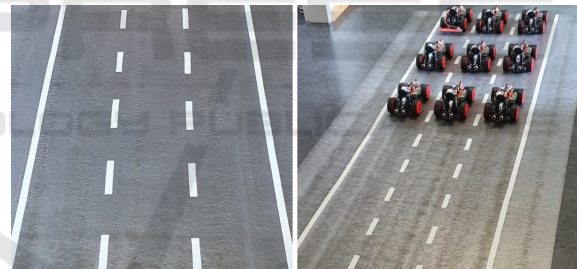
Figure 3: Construction of the three-lane model motorway. Left: Motorway without model cars. Right: Motorway with model cars.
