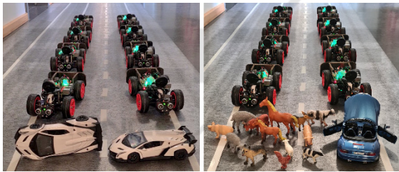
Figure 6: Successfully established emergency corridor in the event of an accident on a two-lane motorway. Left: Car accident. Right: Animals crossing.
