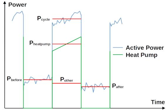
Figure 2: Estimation of the heat pump cycle power  $P_{heat\ pump}$ . The power consumed by all the other appliances  $P_{other}$  during the heat pump cycle is estimated as the average of  $P_{before}$  and  $P_{after}$ .  $P_{other}$  is then subtracted from the average power of the given cycle  $P_{cycle}$  to provide the estimation of  $P_{heat\ pump}$ .
