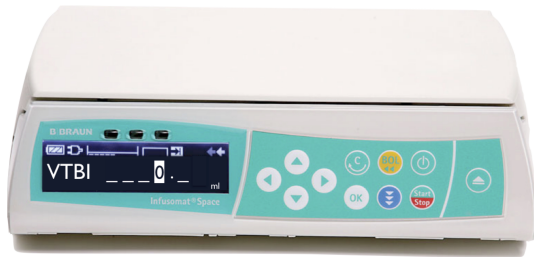
Figure 5: A BBraun Infusomat simulation, set up for start of the interaction sequences shown in figures 6 and 7. ('VTBI' means volume to be infused).
