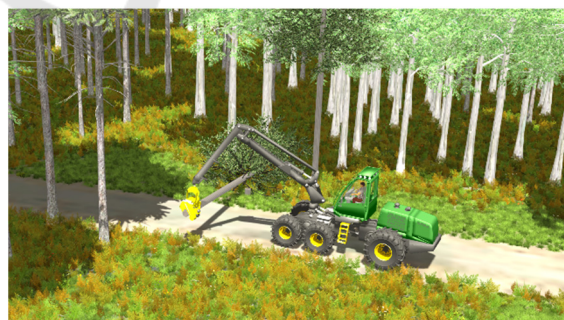
Figure 5: DT of a harvester in a forest environment cutting a tree.
