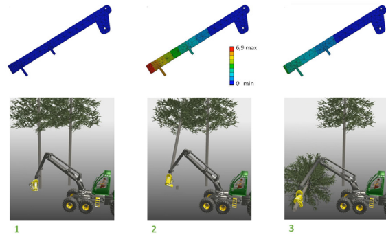
Figure 7: The upper row shows different deformations of the crane arm. As this was an exemplary study, the results are qualitatively and not absolutely. The time points 1, 2, 3 from Fig. 6 can be directly assigned to characteristic actions of the harvester and the resulting deformations of the crane.
