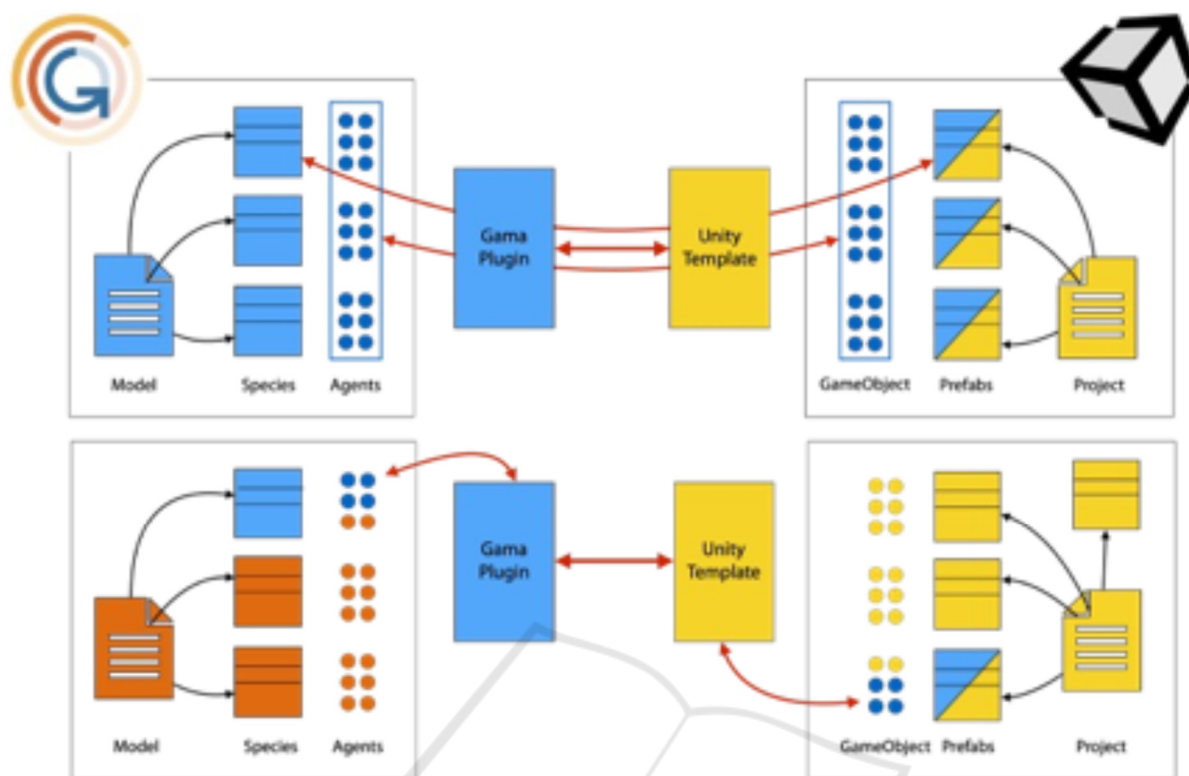
Figure 1: Coupling is based on the definition of a plugin (on the GAMA side) and a model (on the Unity side). This combination allows a wide range of configurations, from bijection (top) to incomplete projection (bottom), to the simple exchange of data between the platforms.
