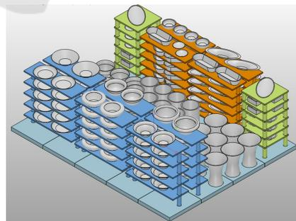
Figure 6: An illustration of the ceramic kiln loading according to the best solution based on the proposed multi-objective algorithm.
