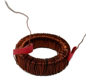
Figure 4: Samples of rail rings with coils wrapped around them.
