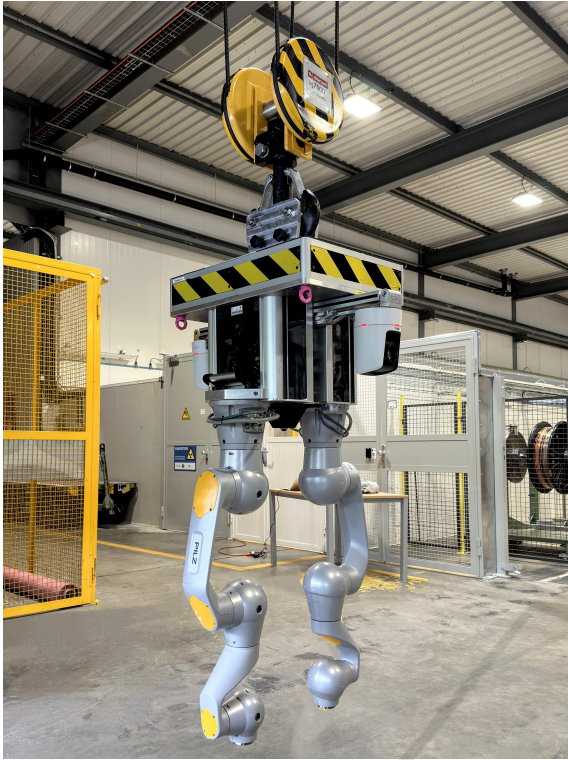
Figure 1: CRANEBot, crane-suspended robotic system in its dual-arm configuration.
