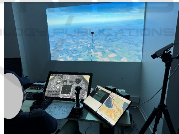
Figure 3: Pilot's workstation including the cockpit, the static HMI CROP and the geospatial HMI CROP.
