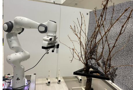
Figure 2: Experimental setup composed of the robot Franka Emika, the Realsense camera D405 and one vine branch.
