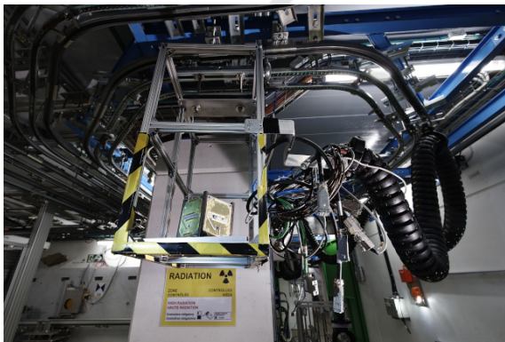
Figure 1: Radiation testing of CELESTA satellite in CHARM facility (CERN, 2024a).
