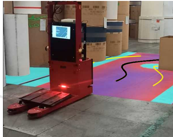
Figure 3: Forklift robot navigating in the printing plant.
