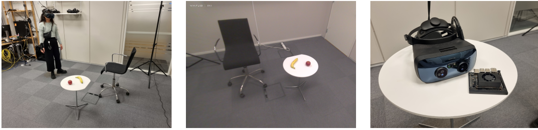
Figure 4: (Left): Experimental setup of our scene. A user is scanning the scene with a Varjo XR-3. (Mid) Example screenshot from the Varjo XR-3 view where the three detected objects are present. (Right) The Varjo XR-3 is tethered, but future generations of XR hardware could (at least mechanically) fit more powerful hardware such as the Jetson Xavier NX 8 GB.
