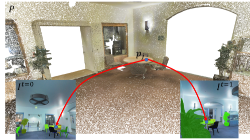
Figure 2: 2D-3D correspondences between images (with instance semantic masks visible) and point cloud from the Lounge 2 of the S3DIS dataset. We will use a heavily down-sampled point cloud, only keeping 0.3 % of the points, in order for us to work on XR devices.
