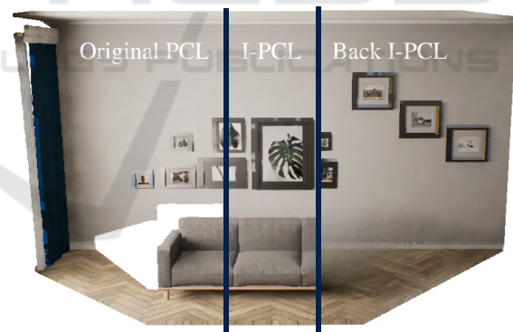
Figure 1: Rendered Point Cloud of 3D Scene with Occlusion, Non-Occlusion and Reconstructed Background: The original point cloud (PCL), on the left, contains white areas which convey the occlusion problem. The center illustrates the result of the inpainted point cloud (I-PCL) reconstructed using our D-LaMa model. The sofa can be hidden by combining PCL and I-PCL. The reconstructed backside is demonstrated on the right.
