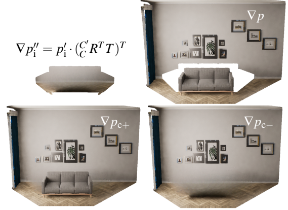
Figure 7: Reconstruction of Inpainted Point Cloud (I-PCL): Top left shows the re-occluded background of the inpainted point cloud \nabla p_i'' generated by the D-LaMa model. The point cloud of the entire scene \nabla p_i'' can be reconstructed as an occlusion-free point cloud \nabla p_{c+} or an occlusion-free point cloud with hidden object \nabla p_{c-} .
