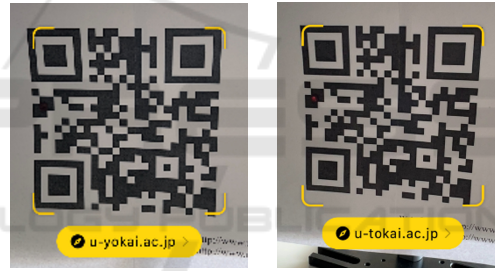
Figure 8: Normal QR code. Figure 9: Wavelength 635 nm (irradiation range 2 mm, illumination power 7.1 mW).
