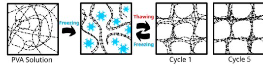
Figure 1: Effect of cycling on the microstructure of PVA-C.
