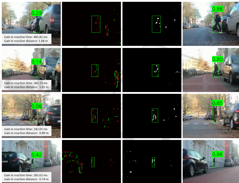
Figure 7: Detection result of low-latency fusion. The first column is the first detection of the fusion method and the last column is the first detection of YOLO v4 detector. The second and third columns are the raw event frame and the background removal result by our proposed method. The confidence score is shown above bboxes. The confidence score threshold for Yolo v4 to accept a detection is 0.8.
