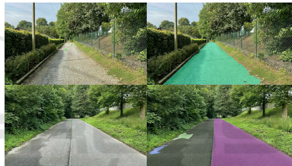
Figure 3: Failure Case Examples: The left column shows the input image with the road obstacles highlighted in green bounding boxes, and the right column shows scenarios where the masks generated by SAM miss detecting the road obstacle as a separate segment.
