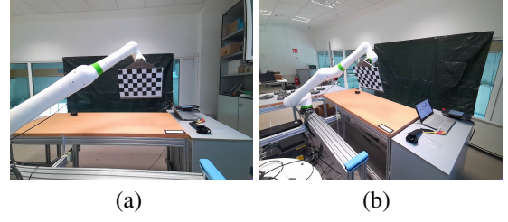
Figure 3: Frame with the calibration pattern acquired by the (a) frontal and (b) lateral camera, respectively.
