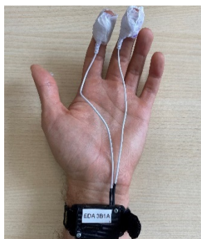
Figure 2 : Sensor and positioning of electrodes on the hand.
