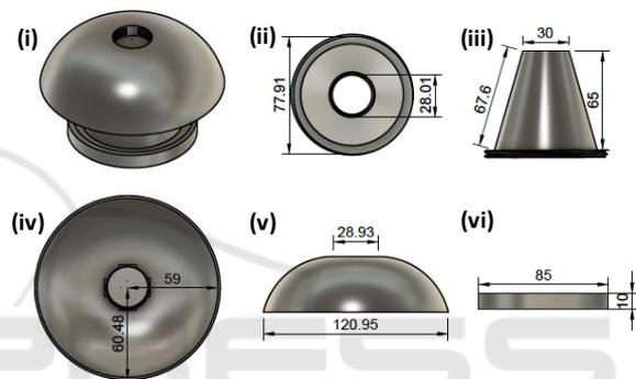
Figure 2: 3-D CAD files showing the, (i) overall structure of the Agri-cone, (ii),(iii) the structure of the conical body and (iv),(v),(vi) the hemispherical top.
