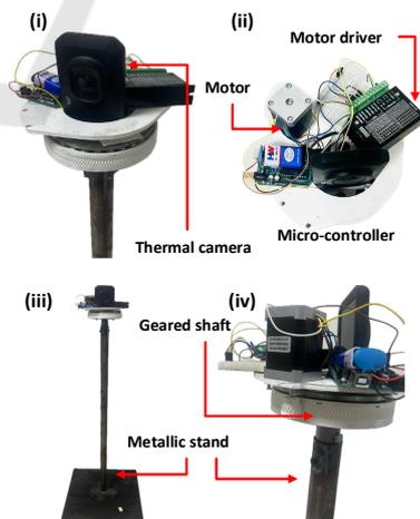
Figure 4: Structure of the Centralised Camera stand along with the various components mounted on it.
