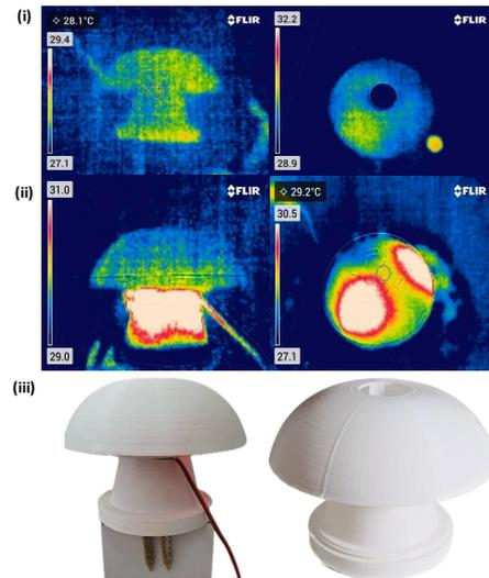
Figure 7: Thermal image of the Agri-Cone when it is (i) switched off, (ii) switched on and (iii) the corresponding original color image.
