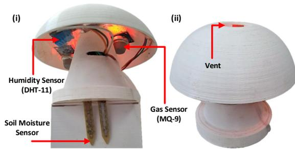
Figure 3: The Agri-cone, (i) Bottom view and (ii) Front view.
