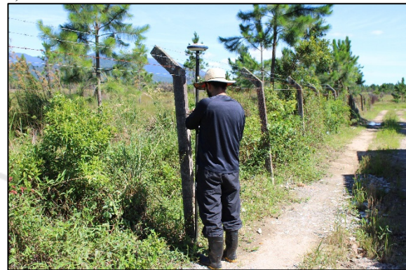
Figure 4: In December 2023, several remaining fragments of the Park's fence were visited. The precise planimetric coordinates of various points representing the geometry of the fence were recorded.
