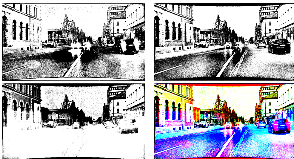
Figure 4: Example of intermediate fused image output from MEFA module combined with RT-DETRv1 model. Grayscale images correspond to a specific single channel of the color image.
