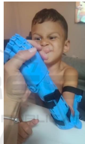
Figure 3: Prosthesis designed for a child with a transradial amputation.
