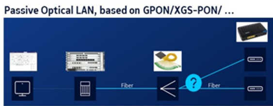
Figure 4(a): G-PON used for a Passive Optical LAN.
