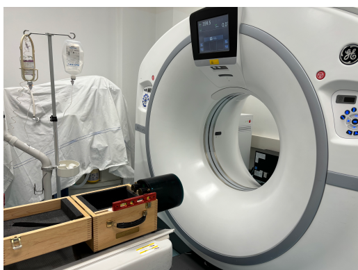
Figure 2: Catphan-500@ phantom acquisition setting. The phantom is placed on its case leveled and aligned with the scanner alignment markers.
