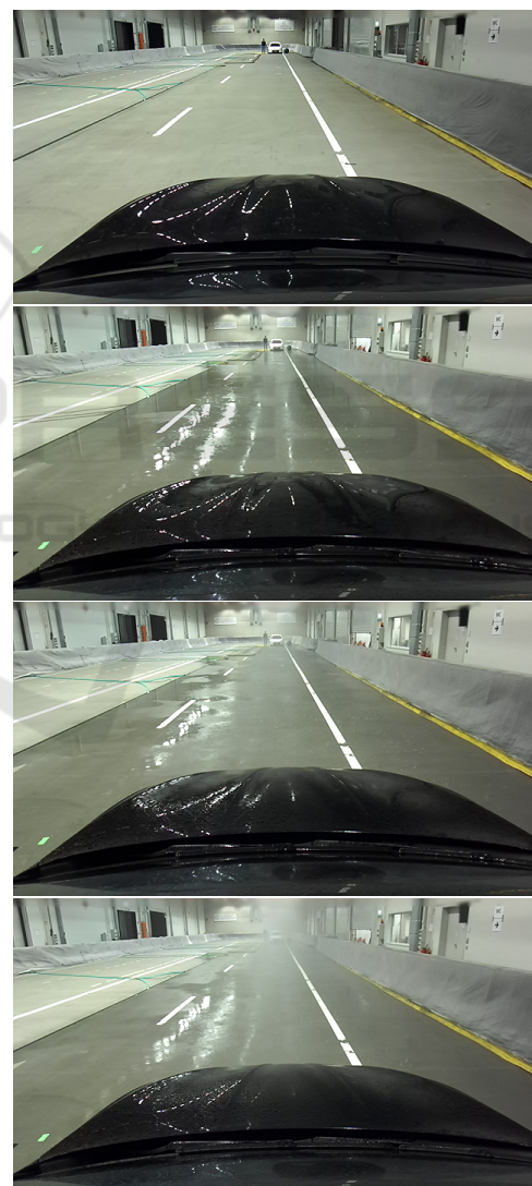
Figure 9: From top to bottom: Target objects positioned 50 meters from the sensors in dry conditions, and during rain precipitation of 20, 60, and 100 mm/h.
