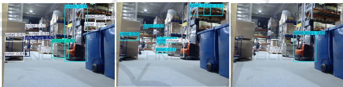
Figure 4: Comparative detection results for 480p image. YOLOv8n a detected a pallet truck as a forklift.
