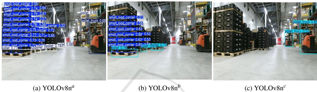
Figure 3: Comparative detection results for 1080p image. YOLOv8n c gave best performance to detect pallet trucks.
