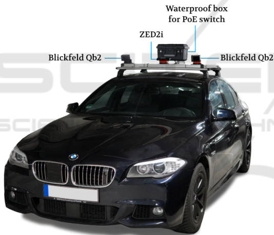
Figure 1: Sensor setup on a test vehicle, featuring two Blickfeld Qb2 LiDAR units, a ZED2i stereo camera, and a waterproof box for PoE switch mounted on the roof.
