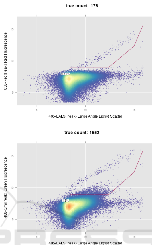
Figure 7: Automated (five-sided) gating results for two different markers showing accurate predictions of the gating boundaries.
