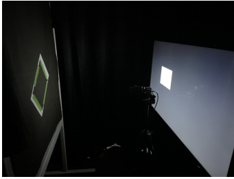
Figure 3: Imaging environment with display as light source.
