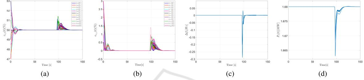
Figure 4: Resilience analysis via LHS method in uncertain delays conditions with  $\tau^* = 0.1$  [s]. Time-history of: a)  $\epsilon_{i,1}(t)$  [%],  $i \in \mathcal{V}_{N_1}^c$ ; b)  $e_{\epsilon,i,1}(t)$  [%],  $i \in \mathcal{V}_{N_1}^c$ ; c)  $\Delta f_1(t)$  [Hz]; d)  $P_1(t)$  [MW].
