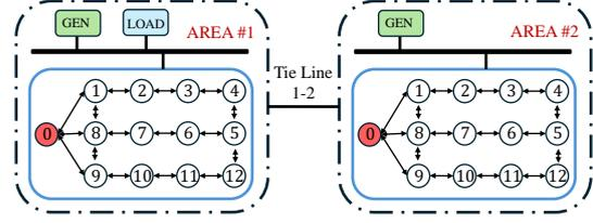
Figure 2: Communication and electrical topologies of 2-Area power System.
