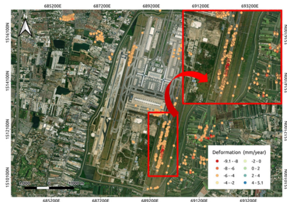
Figure 9: A subsidence rate map of Suvarnabhumi Airport, focusing on the runways and taxiways that require special attention, derived from time-series InSAR processing.
