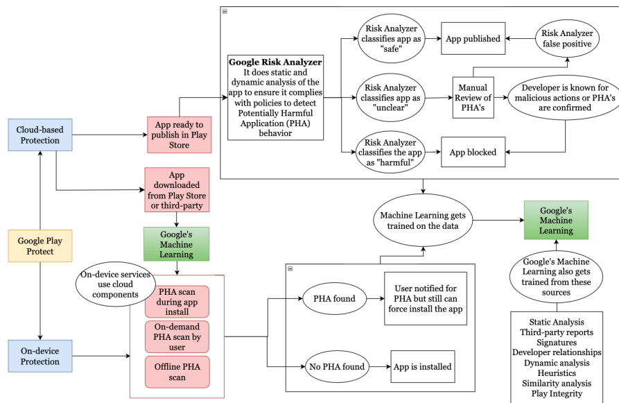
Figure 1: A high-level overview of Google Play Protect showing how Google uses Static Analysis, Dynamic Analysis, and ML techniques together to analyze apps for malicious behavior.
