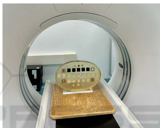
Figure 5: Custom phantom acquisition setting. The phantom is placed with its base on the wooden slab leveled and aligned with the scanner alignment markers.
