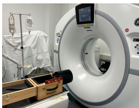
Figure 4: Catphan-500® phantom acquisition setting. The phantom is placed on its case leveled and aligned with the scanner alignment markers.
