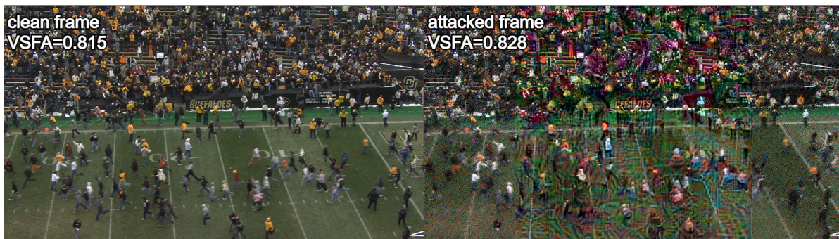
Figure 4: Example of IC2VQA attack. Cross-layer loss is computed for layer1 of SPAQ, \epsilon is set 50/255, number of iterations is set to 20. The visual quality of clean video is obviously higher than that of the attacked video, however, VSFA metric rates the attacked video as having higher quality.
