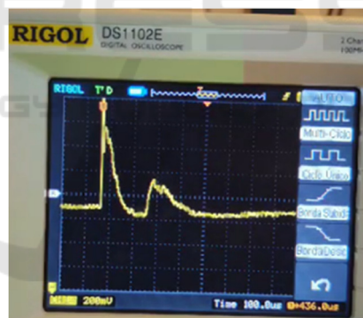
Figure 4: Photoacoustic signal recorded by an oscilloscope.
