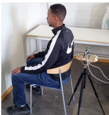
Figure 1: Experimental setup with the radar sensor placed behind the participant.
