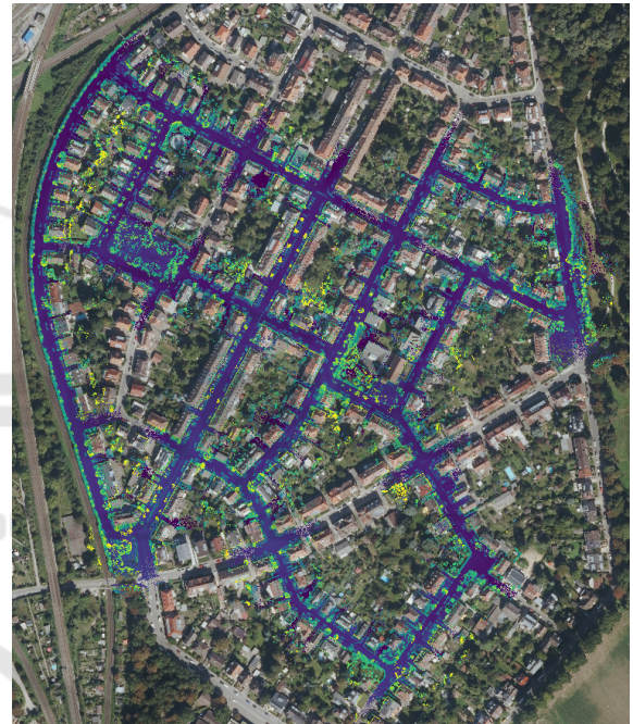
Figure 7: KITTI Seq. 00 point cloud map, created with our approach, plotted to the orthophoto of Karlsruhe.
