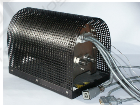
Figure 3: External high temperature density measurement cell (Anton Paar GmbH, 2005)
