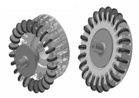
Figure 3: The explosive view of new omni directional wheel and Omni directional Wheel
