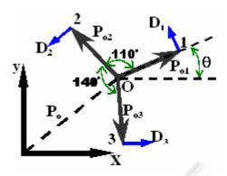
Figure 5: Omnidirectional Robot Model, Top View.
