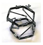
Figure 1: A Stewart-Gough platform model constructed using Lego
