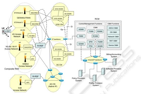
Figure 1. The RMP in a Beyond 3G mobile network architecture.
