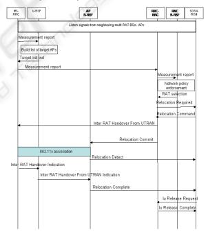
Figure 4: Handing over a connection from UMTS to WLAN
