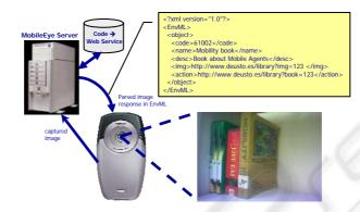
Fig. 3. MobileEye application architecture.
