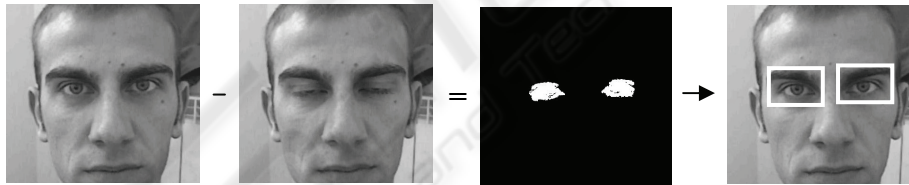
Fig. 3. Blink detection. The first two images represent two consecutive frames of a blink. A difference image is then created. An appropriate filtering enhances the zones where a high changes of intensity occur, i.e. the eye regions.
